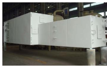
The SR Series Nitrogen Generator is a modular, "packaged" type plant furnished in four preassembled modules: feed air compressor, air chiller, pre-purifier and cold box. Standard models are available with production capacities of 500 to 1000 Nm<sup>3</sup>/hr.
