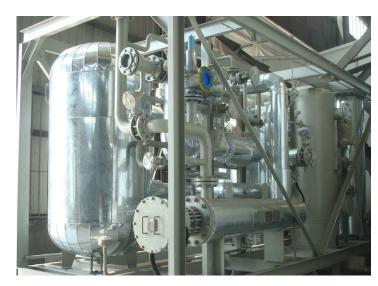
The LA Series Nitrogen Generator is a "liquid assist" type system wherein process refrigeration is supplied by a small external source of liquid nitrogen instead of by expansion, thereby eliminating the need for a turboexpander. This process is especially attractive where liquid backup is required. The plant is a modular, "packaged" type plant furnished in four preassembled modules: feed air compressor, air chiller, pre-purifier and cold box. Standard production capacities: 500 to 1000 Nm3/hr.
